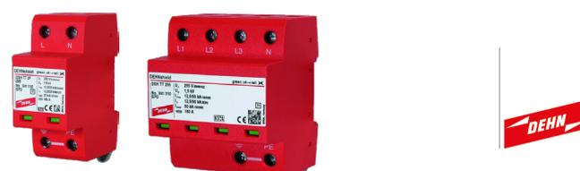
Suitable for TN-S & TN-C-S (PME) earthing systems / For installations with lightning protection system (LPS 3 & 4) or for an overhead supply line / 25/50kA / Protects against surges and from direct lightning strikes / For domestic, commercial & light industrial applications typically up to 125A
